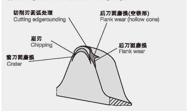
滚刀刀齿的磨损形式 Typical signs of wear on the cutting edge
