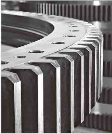
用于外齿轮粗开毛坯的粗铣刀 Coarse roughing of external gears
