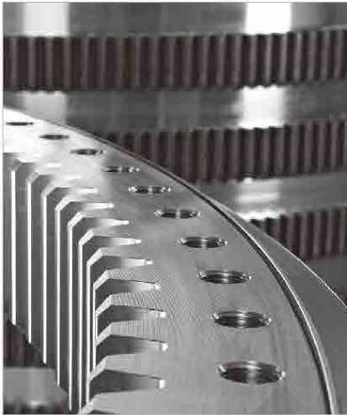
用于内齿轮粗开毛坯的粗铣刀 Coarse roughing of internal gears
