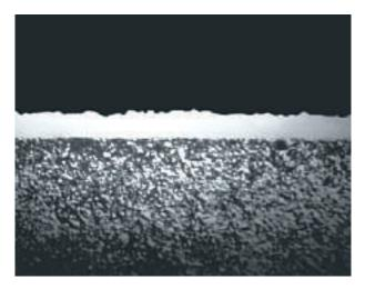
Cross-section of ATCoat coating
