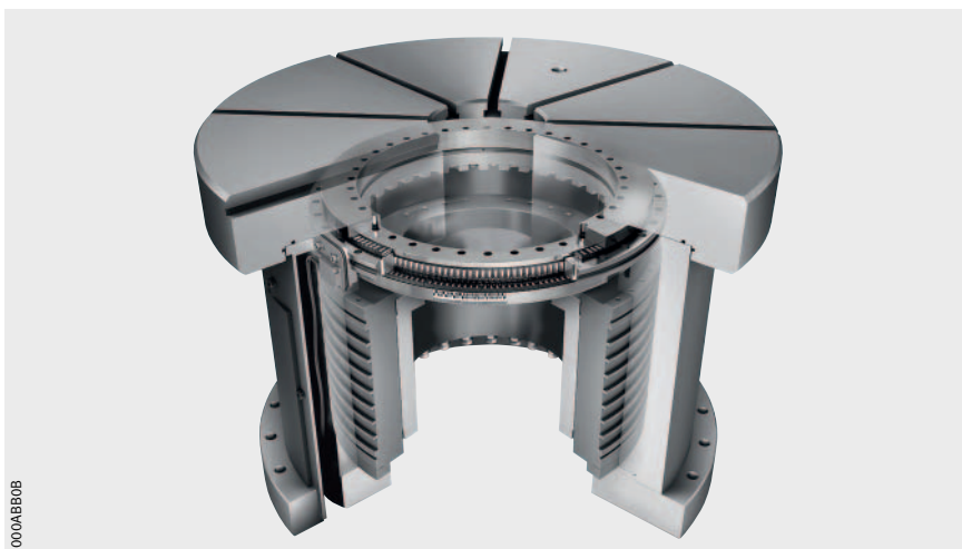
Figure 5: Easy-to-mount rotary table assembly with axial/radial bearing YRTCMA, easily accessible measuring head, no adjustment of measurement gap in fitting or replacement
